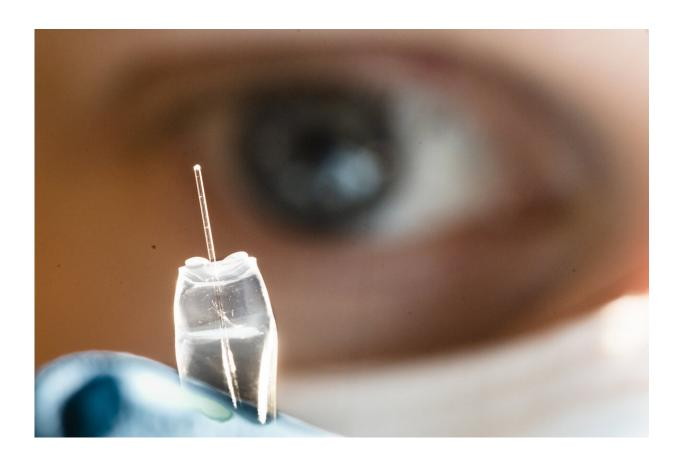
An ion pump can deliver cytostatics more accurately in the brain, which gives less severe adverse effects in chemotherapy. Credit: Thor Balkhed
