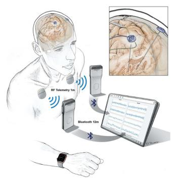
Implanted electrodes stream recorded data to a pocketsized device worn by a patient. The data are then wirelessly transferred to a tablet and then uploaded to the cloud via a HIPAA-compliant server. Credit: Starr lab, UCSF
