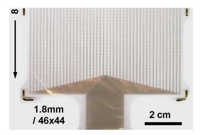
Image of one of a flexible mats of closely spaced sensors being developed at UC San Diego. These kinds of sensor grids are temporarily placed directly on the surface of the brain during some cancer and epilepsy surgeries. Credit: University of California - San Diego
