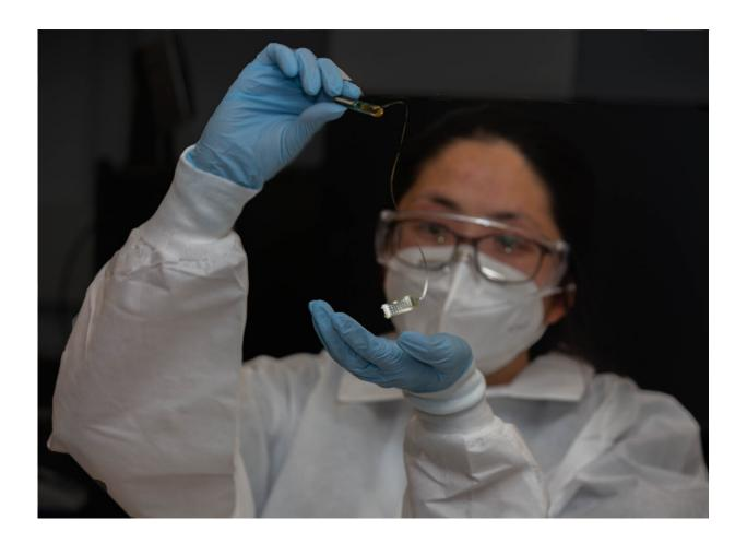
Due to their high-density grid layout, small size and their ability to conform to the hippocampal surface, the LLNL-developed micro-electrode arrays provided researchers with a critical "birds-eye-view" of how traveling waves moved and reversed over the surface of the hippocampus. Credit: Lawrence Livermore National Laboratory
