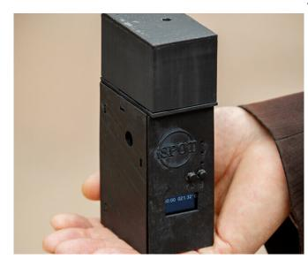
Researchers have developed a new approach to coronavirus testing, creating the first hand-held, battery-powered testing device that can yield accurate results in half an hour. The device can simultaneously test for multiple genes, researchers report. Credit: L. Brian Stauffer
