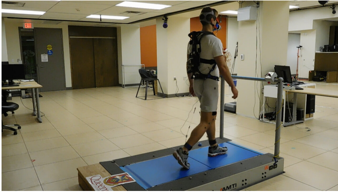
Soft exoskeleton on treadmill. Credit: Queen's University Faculty of Engineering and Applied Science
