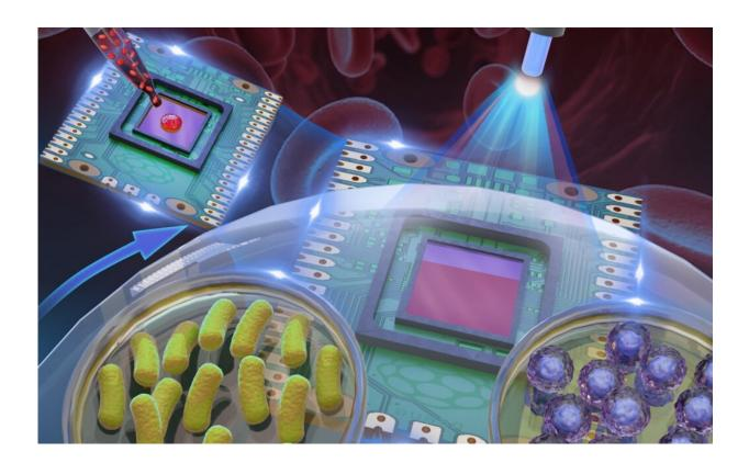
Blu-ray microscope with blood-cell lens. The scheme of the microscope device modified from a Blu-ray disc. A monolayer of blood cells was smeared on top of the image sensor as a high-resolution computational lens with a theoretically unlimited field of view. Credit: Guoan Zheng
