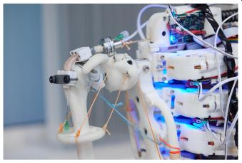
Humanoid bioreactor platform developed to provide engineered tendons with human-like mechanical stimulation. It consists of a robotic shoulder combined with a soft bioreactor chamber. The small chamber, positioned at the supraspinatus tendon location, contains human cells grown onto a biomimetic material and is filled with culture medium. Credit: Fisher Studios
