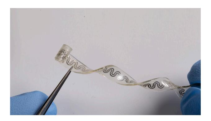
The soft flexible device bends and stretches with the body, without the need for bulky, rigid hardware. Credit: Northwestern University
