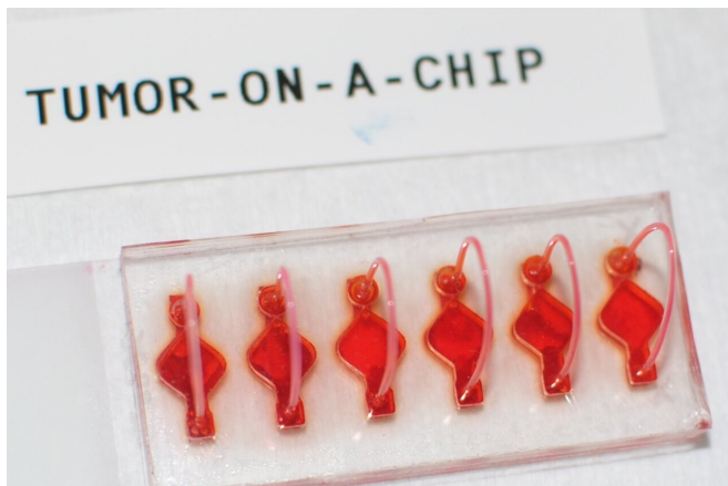
WFIRM's tumor-on-a-chip system is used to test drug treatments. Credit: WFIRM
