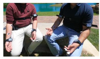
Wearable devices that collect electrodermal activity (like the research devices above) can be used to accurately (and almost instantaneously) infer important data about the wearer's mental state. Credit: NYU Tandon School of Engineering
