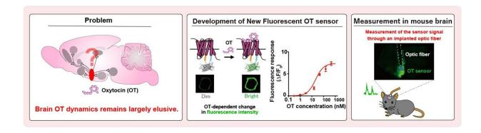
The problem in this research field(left) and approaches to address the problem (center, right) are described. In this study, we developed a fluorescent sensor for real-time measurement of brain oxytocin dynamics in living mice. This new tool will pave the way for the elucidation of how oxytocin acts on the brain during a variety of biological processes. Credit: Daisuke Ino
