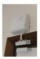
(left) The CASAS Smart Home in a Box (SHiB) contains (middle) passive infrared (PIR) motion detectors coupled with ambient light sensors and (right) magnetic door use detectors coupled with ambient temperature sensors. When there is a change in state, sensors indicate the new state in a text message sent to a central Raspberry Pi. This machine tags the message with the corresponding date, time, and sensor identifier. Credit: *Pain Management Nursing* (2022). DOI: 10.1016/j.pmn.2022.08.011
