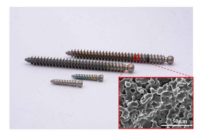
Titanium orthopedic screws with and without silver immobilized onto their implant surfaces using a process developed by Purdue University researcher Rahim Rahimi. Researchers observed that titanium surfaces with laserimmobilized silver had efficient, stable, antimicrobial properties lasting longer than six days. Credit: Rahim Rahimi
