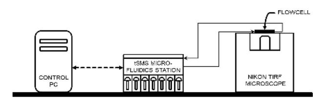
Single-molecule DNA sequencing technical setup. Schematic representation of key instrumentation used to perform single-molecule DNA sequencing. Straight and dashed lines represent microfluidic tubing and electric cables, respectively. Credit: *Nature Biotechnology* (2022). DOI: 10.1038/s41587-022-01447-3
