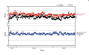
High-content irradiation platform reproducibility for the duration of the profiling effort. The signal-to-noise ratio (SNR), in blue represents the in-plate ratio of radiation survival values between positive control NFE2L2<sup>E79K</sup> (red) and vector (f) control (black) values. The x-axis represents time, delimited by the year of profiling (2017-2019). Credit: *Clinical Cancer Research* (2022). DOI: 10.1158/1078-0432.CCR-22-1914
