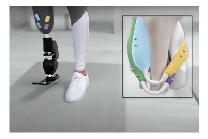
Using a simple set of magnets, MIT researchers have come up with a way to monitor muscle movements, which they hope will make it easier for people with amputations to control their prosthetic limbs. Credit: MIT
