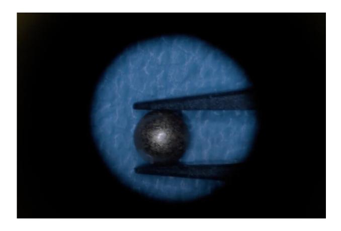
Caption: A small, bead-like magnet used in a new approach to measuring muscle position. Credit: Courtesy of the researchers
