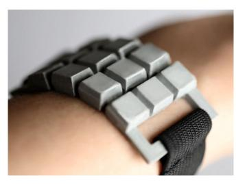
The device is designed to be easy to wear discreetly under clothes. A device attachable to the forearm is one of the possibilities the team is currently exploring. Credit: Juliana Harkki
