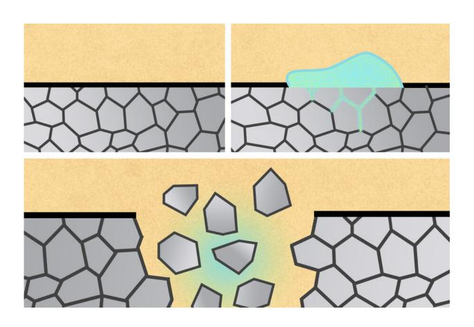
MIT engineers have shown that medical devices made from aluminum can be disintegrated within the body by exposing them to gallium-indium, a liquid metal that seeps into the boundaries between the grains of the metal. Credit: MIT News, based on figures courtesy of the researchers
