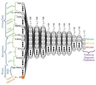
Feed-forward, fully-connected neural network architecture. Nonlinear models have rectified linear units (ReLU) between layers. Final layer implements a softmax. Ll: Number of neurons in layer I. Input features include following. Demog.: Deomographics. Clinical Assess.: Clinical Assessments. Cog. Assess.: Cognitive Assessments. Baseline DX: Baseline Diagnosis. prob.: probability. Credit: *PLOS ONE* (2022). DOI: 10.1371/journal.pone.0277322
