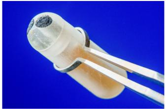
UC San Diego Researchers develop a self-powered ingestible sensor system designed to monitor metabolites in the small intestine over time. Credit: David Ballot for the Jacobs School of Engineering, UC San Diego
