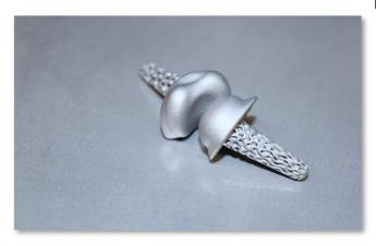
The FingerKIt implants are produced using special 3D printing processes which enable a high level of detail and different surface qualities. Credit: Fraunhofer IAPT
